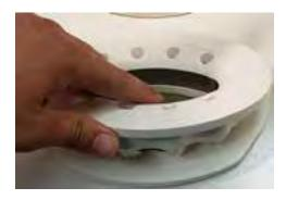
4. Push down on the other side of the insert to seat it against the filter Ifange.
