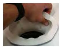
3. Once the one side is released, the filter may need to be tipped back to the other side to release.
