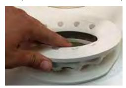
9. Push down on the other side of the insert to seat it against the filter flange.
