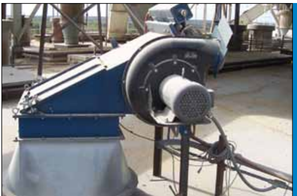
CPV-3 Grain silo bin vent (1200 cfm)
