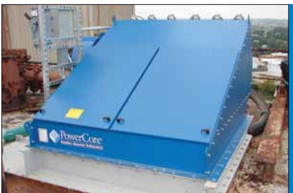
CPV-12 Cement silo bin vent conveyor (3700 cfm)
